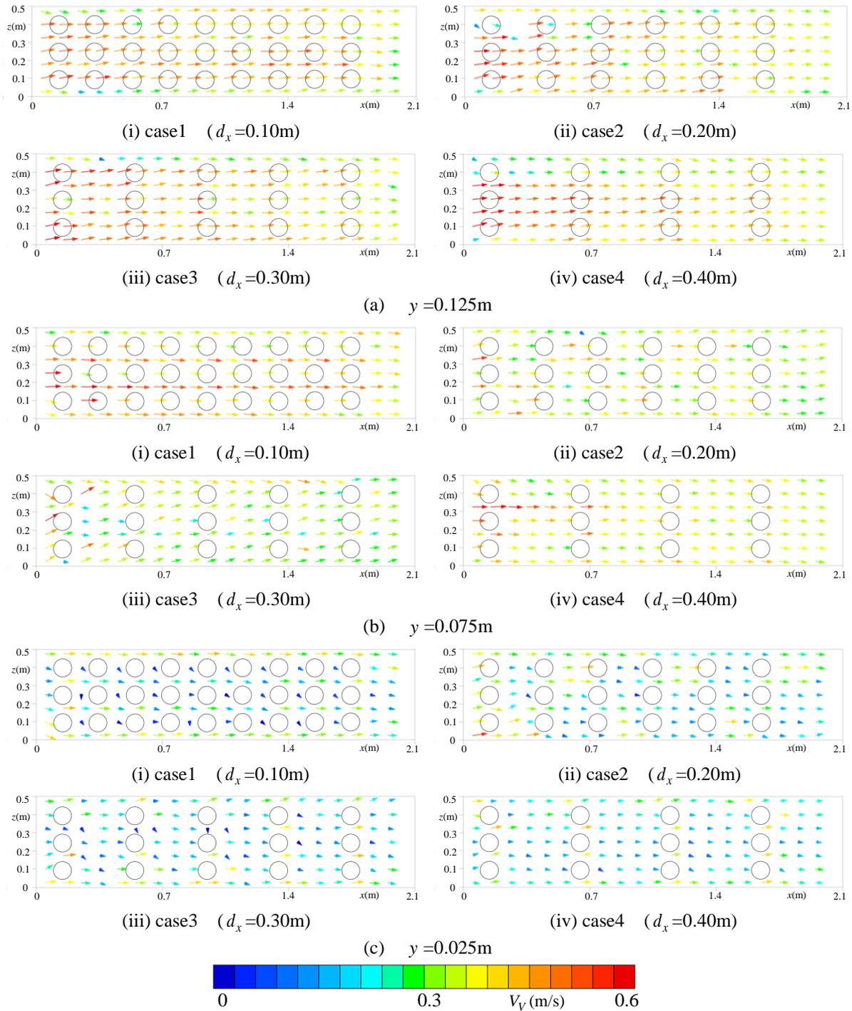
Figure 3. Flow velocity ( $V_V$ ) on each height ( $y = 0.125, 0.075, 0.025\text{m}$ ) of open-channel
